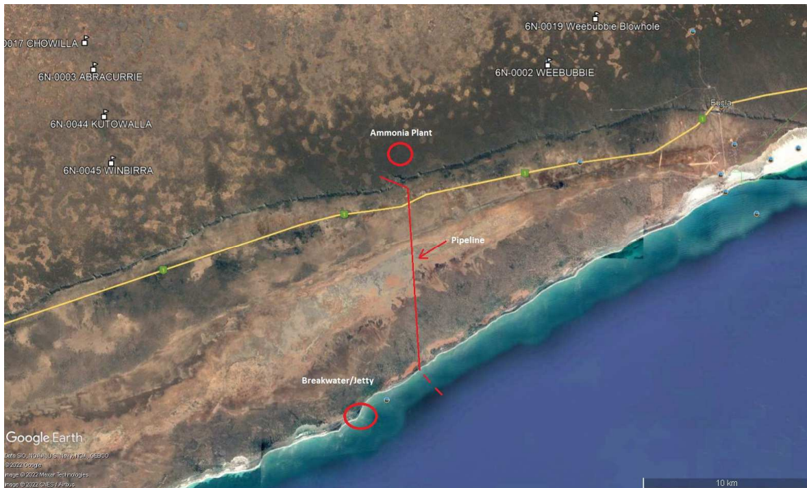
Figure 2: Route of the piping for the ammonia to reach the shipping facilities. Map: Robert Kershaw, prepared for the Conservation Commission, based on information supplied by Western Green Energy Hub, November 2022.
