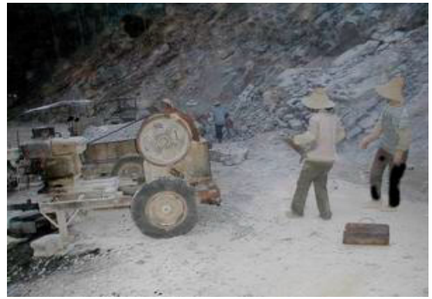
Figure 42: Women quarry workers carrying hand shovel buckets of limestone to a mobile crusher at Quarry Number 2 near Lingyun County town.
