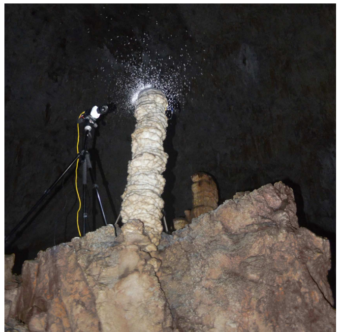
Figure 2. High speed camera set up in the Aven d'Orgnac, France. Note the splash 'umbrella'. Image courtesy of Dr Justine Parmentier.
