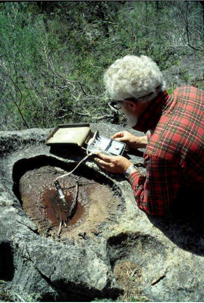
Yarrangobilly, NSW. Joe Jennings measuring the acidity of water in a solution pan . The decaying vegetation will enhance solution.
