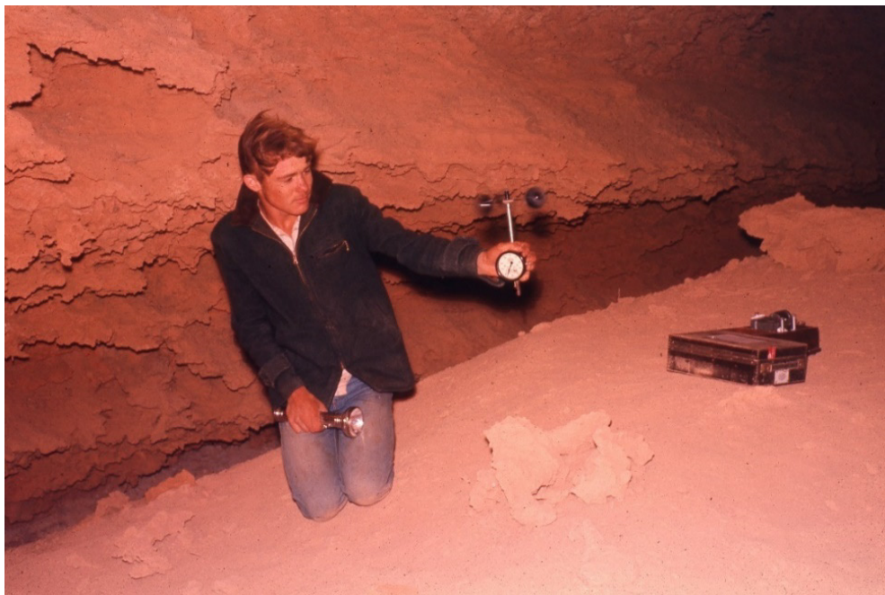
Figure 2: Measuring Southerly Buster airflow
