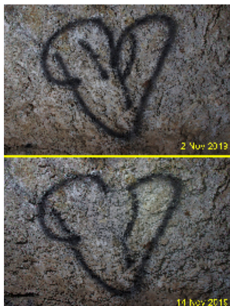
Figure 8- A closeup of a section of graffiti in Figure 6. Slurry mix was applied on 2/11/2019 and allowed to dry for 12 days before taking the second photo
