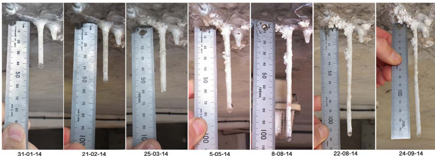
Growth of calthemite straw No.1. The sequence shows the growth of 104mm in 237 days. When there was only one drip every 11 minutes, this straw grew at 2mm per day. The date below each image relates to date of measurement recording.
