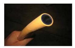
Figure 2- a close up view of the optic fibre showing the polymer core and cave coloured exterior coating.
