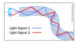
Figure 1 - A diagram showing the transmission of light along an optic fibre by total internal reflection.
