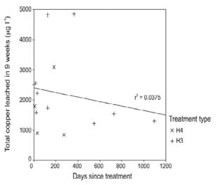
**Figure 5**. Copper leached from treated wood blocks of varying ages in nine weeks. Line of best fit is for H3 timber.
