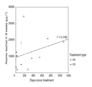
Figure 4. Arsenic leached from treated wood blocks of varying ages in nine weeks. Line of best fit is for H3 timber.
