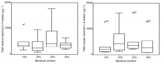
Figure 1. Arsenic and copper leached from treated wood blocks of varying moisture content in nine weeks.
