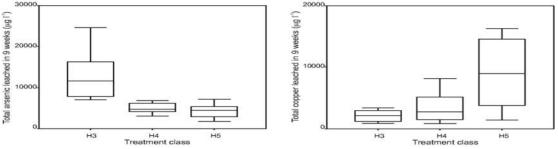
Figure 2. Arsenic and copper leached from treated wood blocks in nine weeks.
