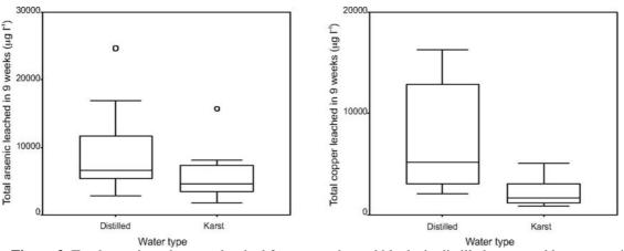
Figure 3. Total arsenic and copper leached from treated wood blocks in distilled water and karst water in nine weeks.
