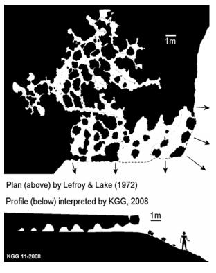
Fig 6: The small laterite maze cave at Chittering, WA. From a map by Lefroy & Lake (1972), a pair of school students who explored and mapped the system as a science project. Ken Grimes has added an interpreted profile. Note the scale bar; many of these passages would be inaccessible to a 'standard-size' adult caver!
